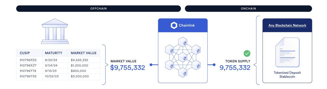
One of the key risks for tokenized assets is the minting of more tokens than the current market value of the offchain collateral. Chainlink PoR can be used to trigger a circuit breaker connected to the minting function of a tokenized asset, which prohibits the minting of more tokens if it determines that the collateral value fell below a certain threshold.
